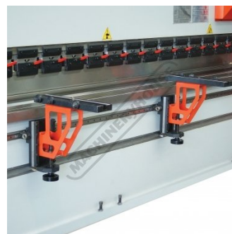
Adjustable and Sliding Front Sheet Supports on Linear Guideways
