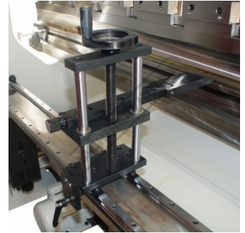
Adjustable R Axis Height with Dial on Linear Guideways
