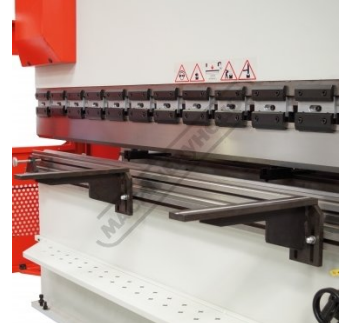
Adjustable and Sliding Front Sheet Supports
