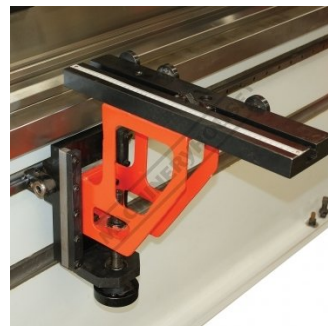
Sheet Support with Scale and Flip Over Stops
