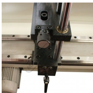
Micro Adjustment Backstop
