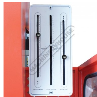
Adjustable Travel Limit Control
