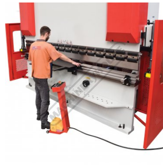
Laser Guarding system In Use
