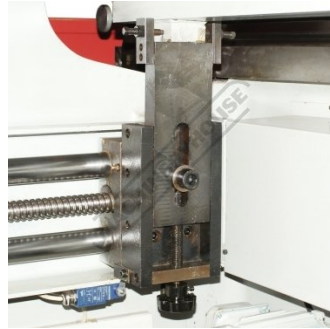
Adjustable Height Ballscrew Backgauge
