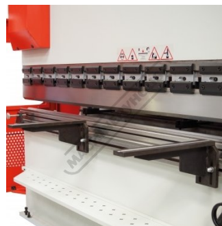
Adjustable and Sliding Front Sheet Supports
