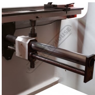
Estun NC E21 Control Ballscrew Back Gauge
