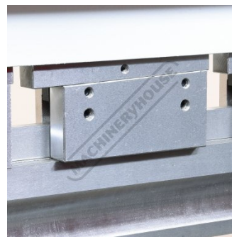
Adjustable Top Tool Taper Wedge System
