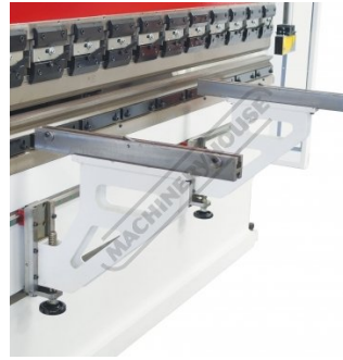
Sliding Front Sheet Supports on Linear Guideways
