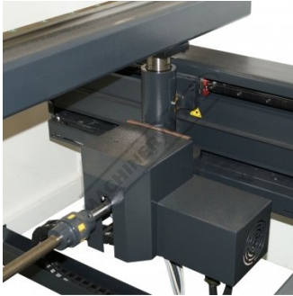
CNC Ball Screw Backgauge with R Axis
