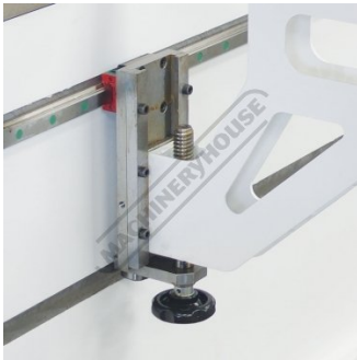
Front Sheet Support Height Adjustment
