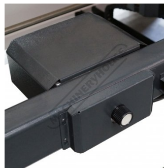
Backgauge Manual Fine Adjustment
