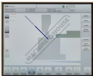
Program Bend Sequence Simulation
