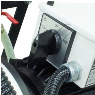
Main Power Switch
