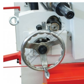
Hand Wheel For Material Thickness Adjustment
