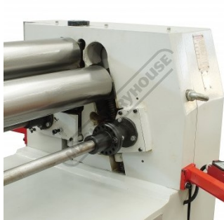
Motorised Up and Down Rear Curving Roller Right Side
