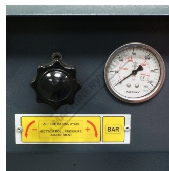
Hydraulic Pressure Plate Clamping Adjustment
