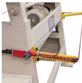
Safety Trip Wire
