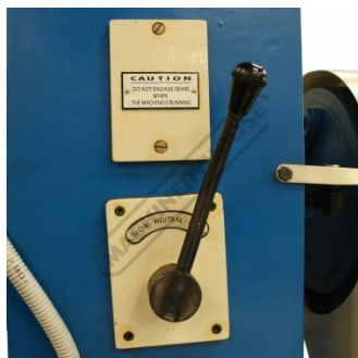
Slow Medium Fast Stroke Speed Lever
