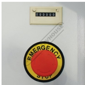
Emergency Stop and Cut Counter
