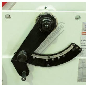
Rapid Blade Adjustment for Material Thickness
