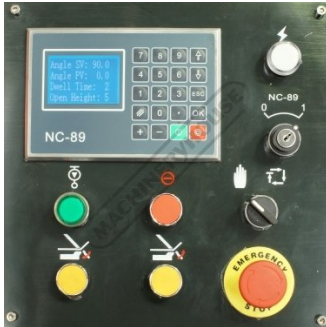
NC 89 Control Panel
