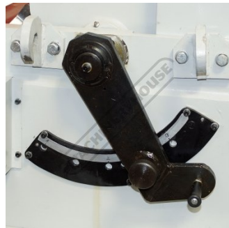
Rapid Blade Adjustment for Material Thickness
