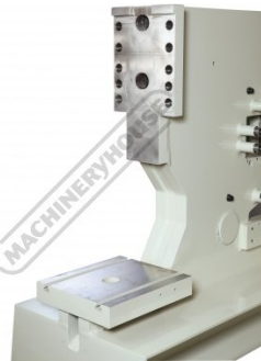
Solid Punching Base With T-Slot Grooves
