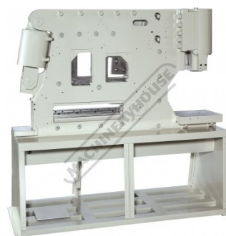
Monoblock Design For Rigid Frame Structure
