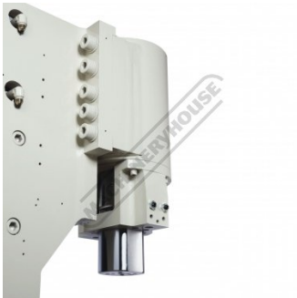
Keyed Punch Ram For Shaped Tool Alignment
