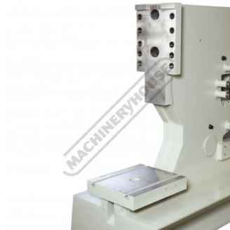
Solid Punching Base With T-Slot Grooves
