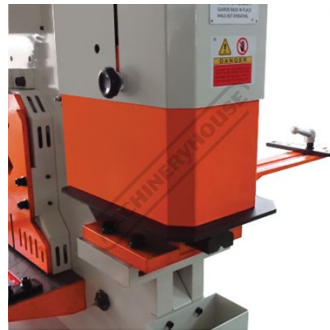
Bending Station Interlocked Safety Cover
