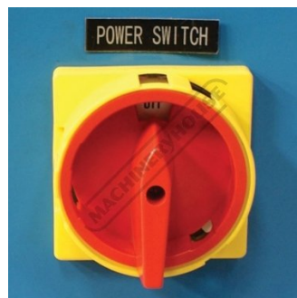
Main Power Switch
