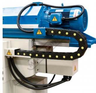
7.5kW / 10hp Spindle Motor
