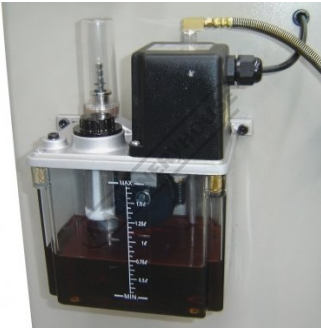
Auto Lubrication System
