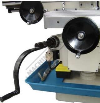
Safety Micro Switch On Z Axis Lever
