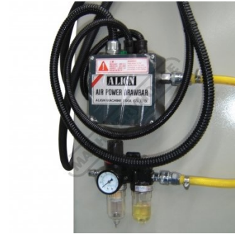
Align Air Operated Drawbar System
