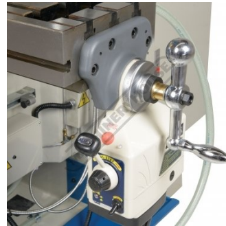
X Axis Power Feed with Rapid
