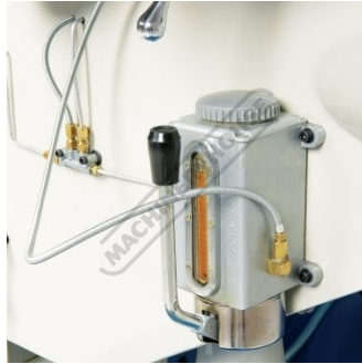
One Shot Lubrication System
