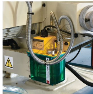
Automatic Slideway Lubrication System
