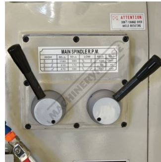
Horizontal Speed Selection Levers
