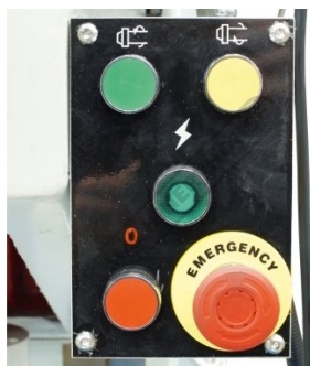
Horizontal Spindle Control Panel
