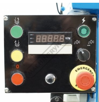
Control Panel with DRO Speed Display
