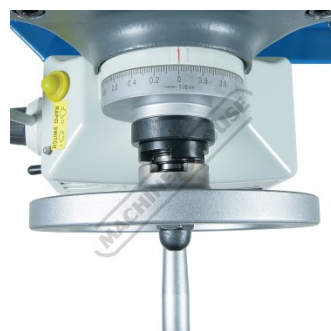
X Axis Dial Power Feed Slide
