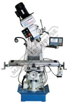
Head Tilts to 45 Deg Left Right
