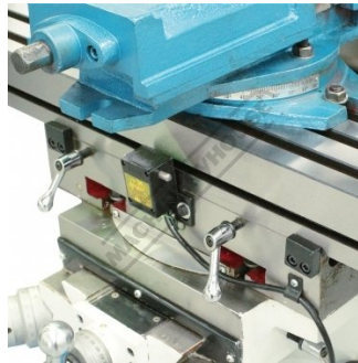
Feed Limit Switches
