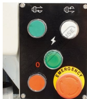
Horizontal Spindle Control Panel
