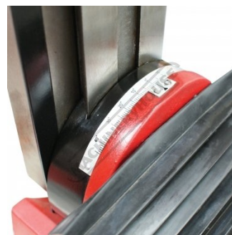
Milling head Tilts 45 Degrees both directions
