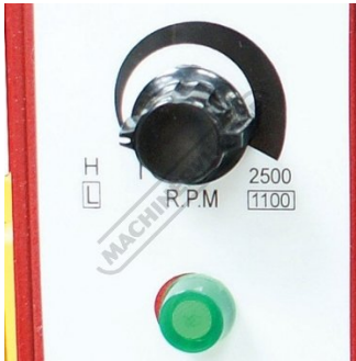
Electronic variable speed system
