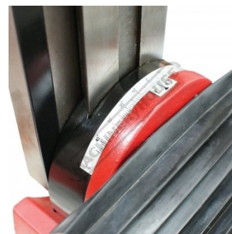
Milling head Tilts 45 Degrees both directions
