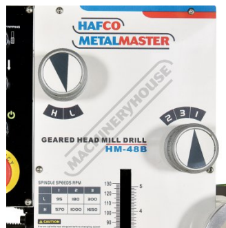
Spindle Speed Controls
