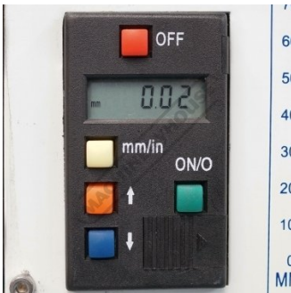
Digital Readout On Quill Depth
