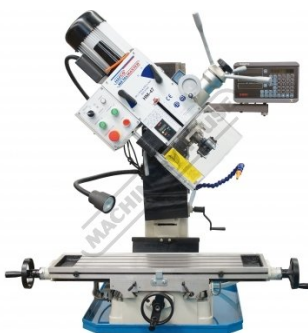
Swivel Head 45 Degrees Front View
