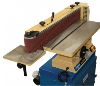
End Table Working Position with Quick Belt Change
