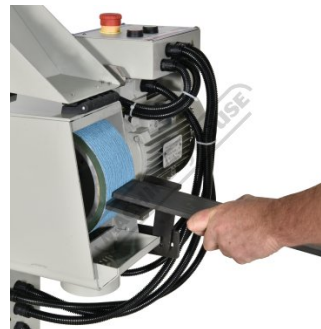
End Station Shown Finishing Flat Bar
