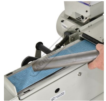
Top Station for Flat Finishing and Deburring
