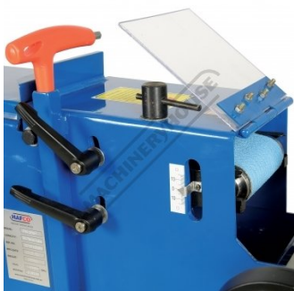
Roller Height Adjustment
