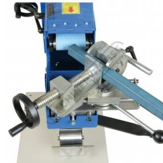
Square Vice Jaws Holding Material at 45 Degrees
