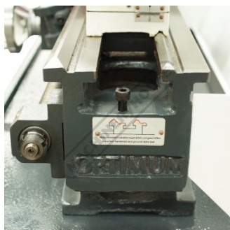
Induction Hardened and Ground Bed
