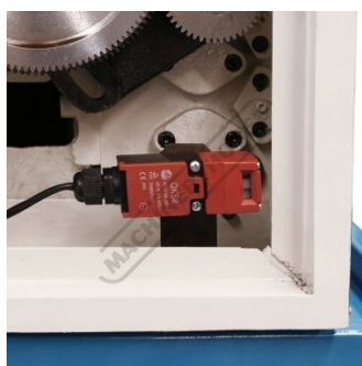
Safety Micro Switch on Side Access Door
