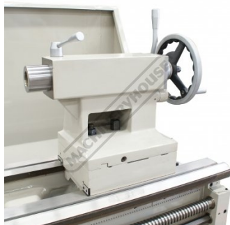
Heavy duty tailstock
