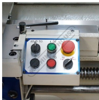
Saddle Switch Board
