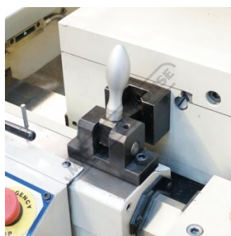
Tailstock Moving Device Locked Position
