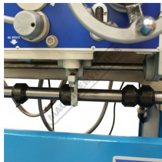
Adjustable 4 position length stop mechanism for accurate repetitive operation
