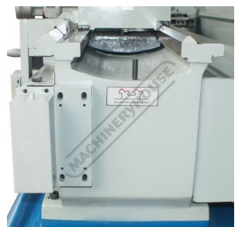
Ground and Hardened Bed
