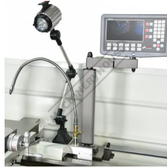
LED Worklight and Coolant Hose
